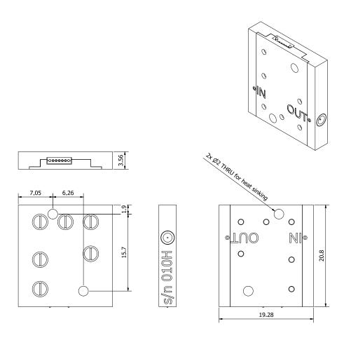
5-pin strip connector seen from outside the LNA (engraved text upward)
