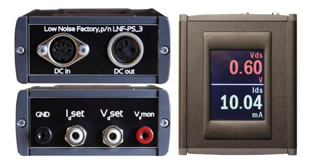
LNF-PS\_3 is a compact power supply designed for LNF's cryogenic Low Noise Amplifiers. The drain voltage is regulated and adjustable within a wide range, and the gate voltage is automatically and continuously adjusted to give a set drain current.
