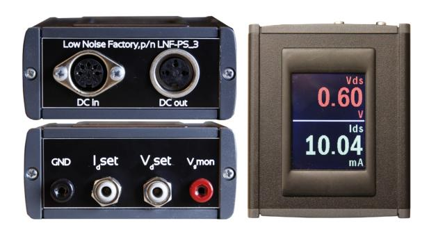
LNF-PS\_3 is a compact power supply designed for LNF's cryogenic Low Noise Amplifiers. The drain voltage is regulated and adjustable within a wide range, and the gate voltage is automatically and continuously adjusted to give a set drain current.
