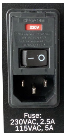
Figure 1 Power Entry Module configured for 230 VAC.
