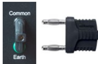
Figure 6 Connecting Common to Earth
