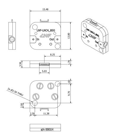
5-pin strip connector seen from outside the LNA (engraved text upward)
