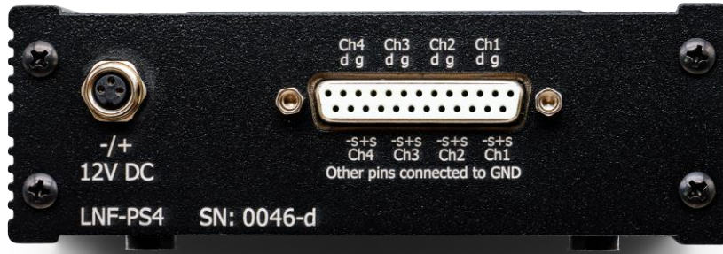
Figure 3 Rear panel equipped with female socket d-sub 25p connector.
