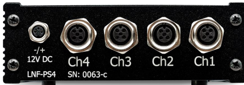
Figure 2 Rear panel equipped with four female socket 5p connectors size M12.
