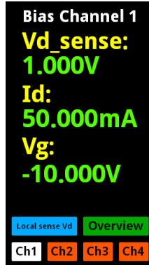
Figure 13 Screen when LNF-PS4 in remote sense mode
